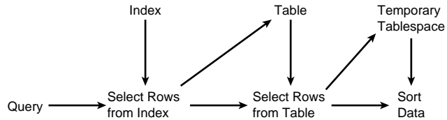
Figure 22.3. Input/output opera- tions and the temporary tablespace.
